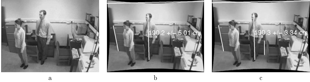
Fig. 17. Measuring heights and estimating their uncertainty, second point of view: (a) Original image; (b) the image has been corrected for radial distortion and height measurements computed and superimposed. With one supplied reference height Z = 190.2 \pm 5.01\text{cm} ( c.f. ground truth value 190cm). (c) With two reference heights Z = 190.3 \pm 3.34\text{cm} . See figure 16 for details.
