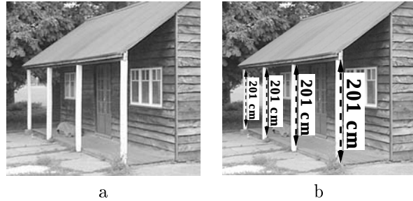
Fig. 1. Measuring distances of points from a reference plane (the ground) in a single image: (a) The four pillars have the same height in the world, although their images clearly are not of the same length due to perspective effects. (b) As shown, however, all pillars are correctly measured to have the same height.
