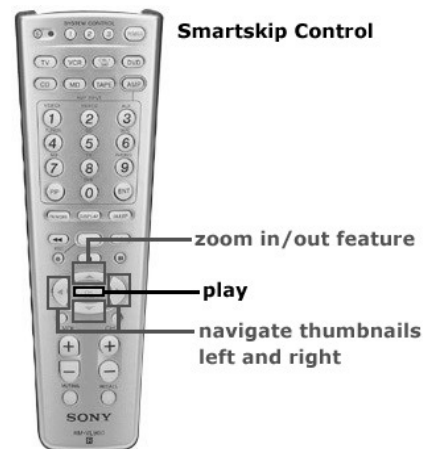
Figure 3: Buttons on a standard Sony Learning Remote Control for controlling SmartSkip (and other interfaces)
