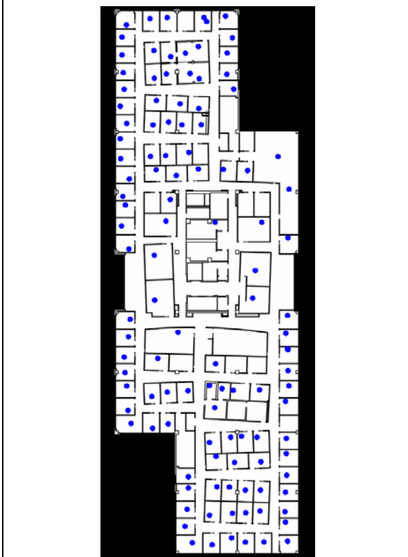
Figure 4: These are the locations we used to test our location algorithm. Altogether we tested on 25,457 signal strength vectors taken at 115 different locations.
