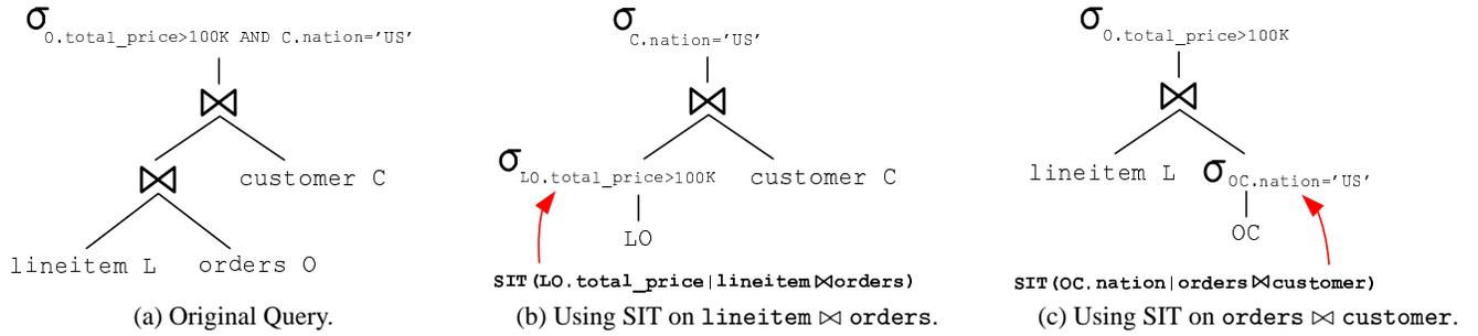
Figure 1: Exploiting SITs using view matching.
