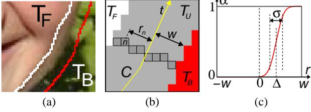
Figure 6: **Border matting.** (a) Original image with trimap overlaid. (b) Notation for contour parameterisation and distance map. Contour  $C$  (yellow) is obtained from hard segmentation. Each pixel in  $T_U$  is assigned values (integer) of contour parameter  $t$  and distance  $r_n$  from  $C$ . Pixels shown share the same value of  $t$ . (c) Soft step-function for  $\alpha$ -profile  $g$ , with centre  $\Delta$  and width  $\sigma$ .
