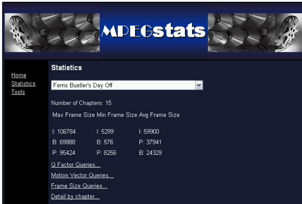
Figure 9 – MPEGstats web interface showing the number of chapters for a title along with the min, max and average frame sizes for I, B and P frames. Links for detailed queries are at the bottom.
