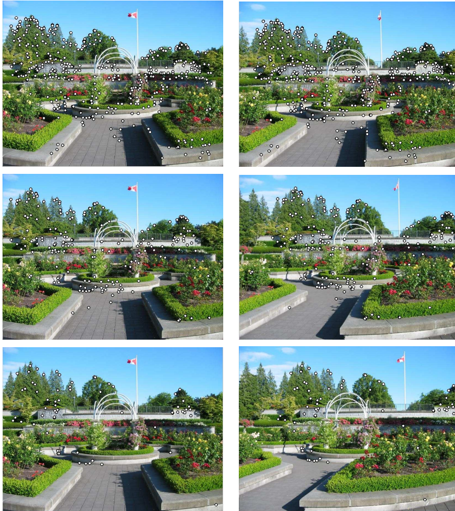
Figure 26: Matching images taken from different viewpoints. Shown are inliers to the fundamental matrix estimated between each pair. The number of matches in each case are 433, 202, 70 with approximately equal increments of 15 degrees between the views. Note that feature matching works well under small viewpoint changes but drops off as the viewpoint change becomes large. This is probably due to affine deformations and partial occlusions.
