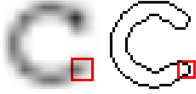
Fig. 1. Features for constructing the spatially-variable filter: a 7x7 patch of the bilinear interpolated image and the corresponding 5x5 patch from the Canny edge image.
