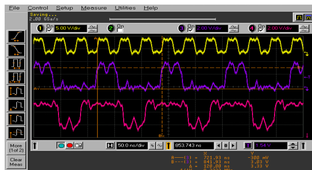
Figure 5. Oscilloscope waveform showing 3 instruction fetch cycles.
