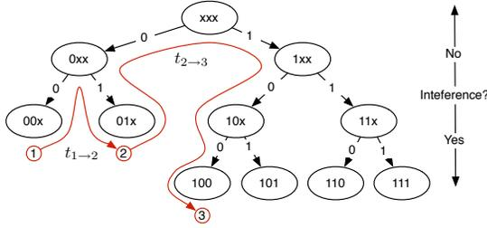
Fig. 4. The anti-collision system. Depending on the tags present in the space, the time taken to traverse the binary tree can vary. Here  $t_{1 \rightarrow 2}$  is faster than  $t_{2 \rightarrow 3}$
