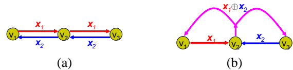
Fig. 1. (a) The conventional solution requires 4 transmissions to exchange two packets between v_1 and v_3 via a relay node v_2 . (b) Using network coding, two packets can be exchanged in 3 transmissions [1].
