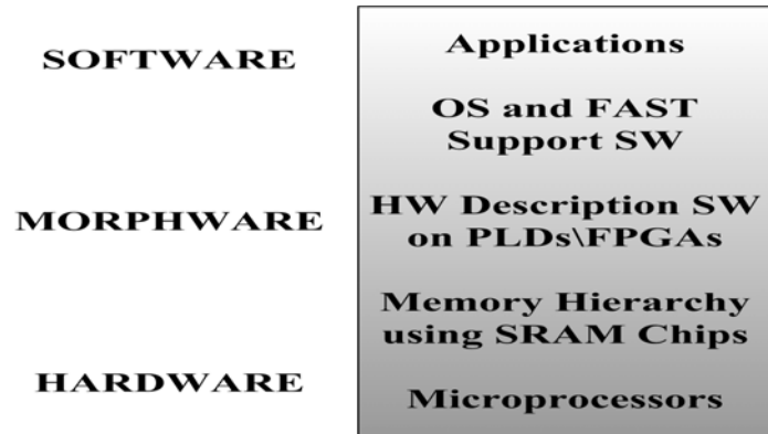
Figure 2.10. All FAST hardware and software components.
