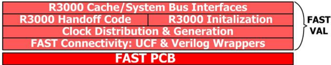
Figure 4.6. The FAST PCB with the Verilog Abstraction Layer components on top.
