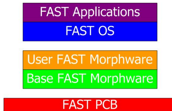
Figure 1.6. FAST system hardware and software stack.
