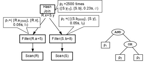
Figure 1. Execution plan and AND/OR request tree.
