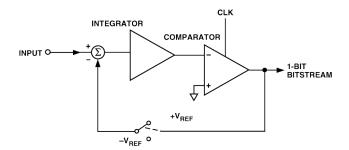
Figure 9: The architecture of a VFC.
