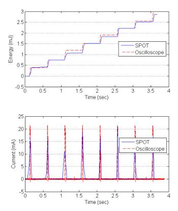
Figure 14: Energy and power tracking of dutycycling TelosB mote using SPOT compared with a digital storage oscilloscope. The flat portions of the top graph represent energy consumed by the mote during sleep while the sharp rises between flat steps represent energy consumed during active cycles. The bottom graph shows the power draw recorded by SPOT by differencing successive energy usage readings.
