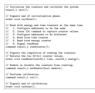
Figure 11: The SPOT application programming interface includes commands to initialize, calibrate, enable, read, and reset the meter.
