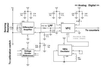
Figure 7: A simplified representation of the analog portion of schematic.
