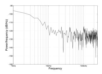
Figure 3: The power spectral density of a node current profile shown in Figure 1.
