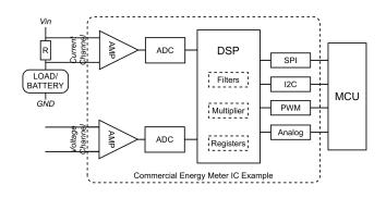
Figure 4: Architecture of a typical energy metering circuit.
