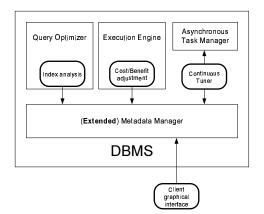
Figure 1: Continuous Tuning Architecture in a DBMS.
