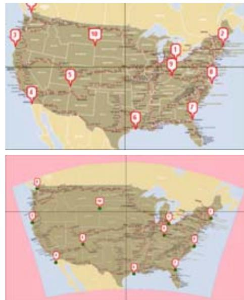
Figure 6. Reprojecting from a conic projection requires bending straight lines.
