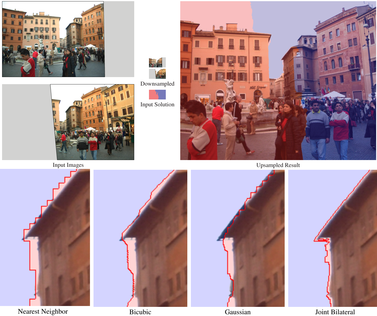
Figure 5: Graph Cut based Photomontage. Upper left: two original aligned images. Upper center: the downsampled images and the resulting labeling solution. Upper right: a composite generated using the JBU-upsampled labeling solution. The label colors are superimposed over the image. The bottom row shows a detail that highlights the advantages of using JBU over standard upsampling methods.
