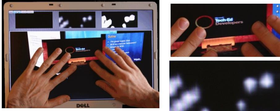
**Fig. 3.** A multi-touch input to the prototype (left). A close-up of the sensor-enabled centre of the display (top right) shows three left-hand fingers held flat against the surface and three right-hand fingertips in contact. The corresponding multi-touch sensor data (bottom right).
