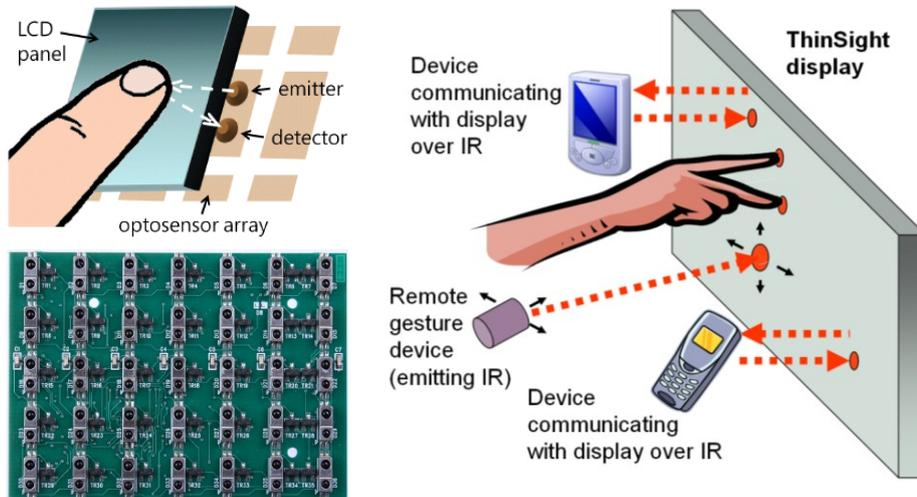
**Fig. 1.** The layout of the ThinSight optosensor array, as it sits behind the LCD panel (top left). The front side of the actual ThinSight PCB, showing the 5x7 array of optosensors (bottom left). ThinSight intrinsically supports multi-touch input, remote gesturing and multiple channels of bidirectional communications, all at the same time (right).
