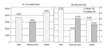
Fig. 6. FPGA area and clock speeds for a  $64 \times 64$  scheduler.
