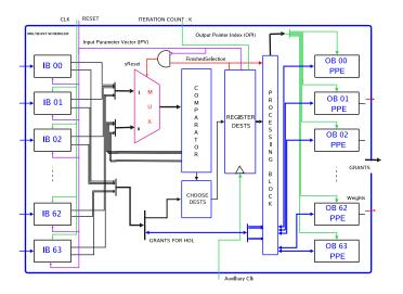
Fig. 5.  $64 \times 64$  WRRM Design Schematic.
