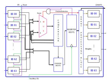
Fig. 4.  $64 \times 64$  Multicycle-WBA Design Schematic.
