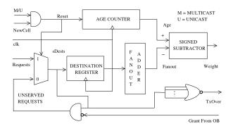
Fig. 1.  $64 \times 64$  WBA Input Block (IB) Design Schematic.
