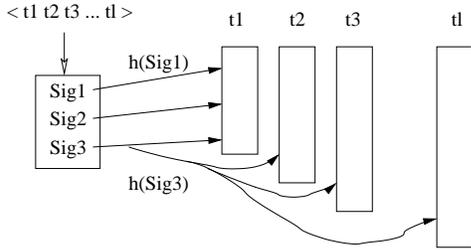
Figure 2: Inverted Signature-based Hashtable
