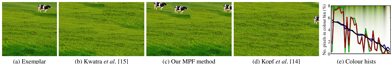
Figure 6. Image synthesis. (a) Input image. (b–d) Larger output images synthesized using (b) the fusion approach of Kwatra et al. [15], (c) our adaption which incorporates a global colour histogram constraint, and (d) the EM-style, global heuristic approach of Kopf et al. [14]. (e) Colour histograms (bins are those used in the global constraint of (c)) for (a) (black), (b) (red), (c) (blue) and (d) (green).
