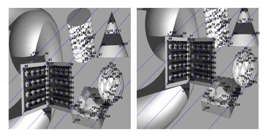
Fig. 23. Scene tracing: The epipolar geometry recovered after discarding outliers and the matched points found using the epipolar constraint
