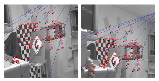
Fig. 16. Scene rotation: Matching result with the relaxation technique and the epipolar geometry recovered using all matched points
