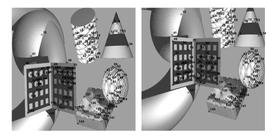
Fig. 21. Scene tracing: Matching result with the correlation technique  $\mathbf{F}$
