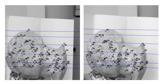
Fig. 8. Scene bust: The epipolar geometry recovered after discarding outliers and the matched points found using the epipolar constraint
