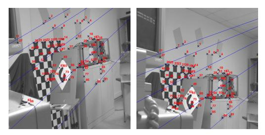
Fig. 17. Scene rotation: The epipolar geometry recovered after discarding outliers and the matched points found using the epipolar constraint
