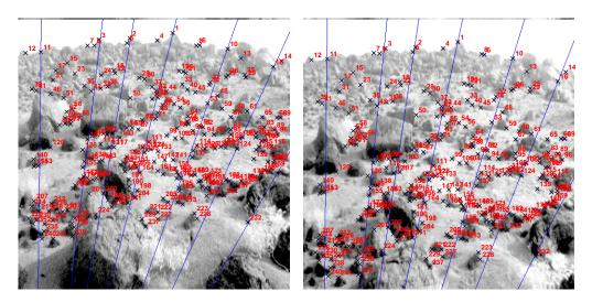
Fig. 14. Scene valley: The epipolar geometry recovered after discarding outliers and the matched points found using the epipolar constraint
