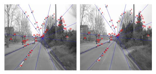
Fig. 11. Scene road: The epipolar geometry recovered after discarding outliers and the matched points found using the epipolar constraint
