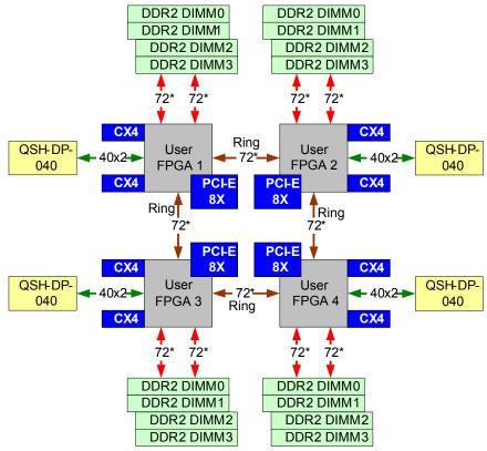
Figure 4. BEE3 main PCB subsystems.
