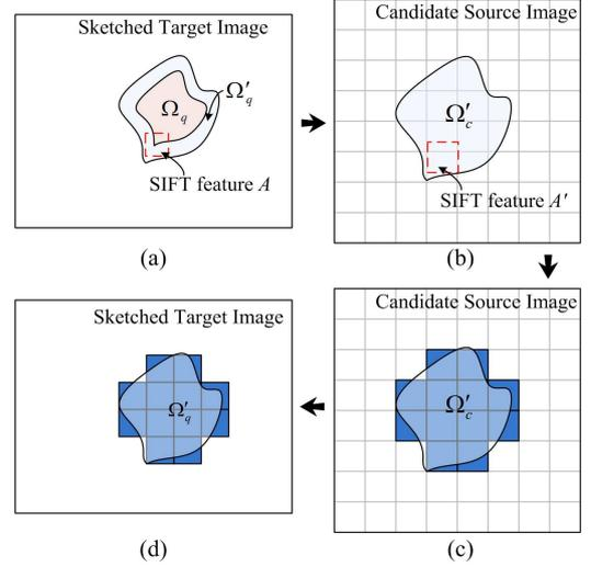
Figure 6: An illustration for gist-based local difference computation. (a) Sketched area in the target image. SIFT feature  $A$  is highlighted using a red dashed box. (b) The corresponding area in the candidate source image. The SIFT feature  $A'$  which is corresponding to  $A$  is also highlighted with a red dashed box. (c) Rasterized area in the candidate source image. (d) Rasterized sketched area in the target image.
