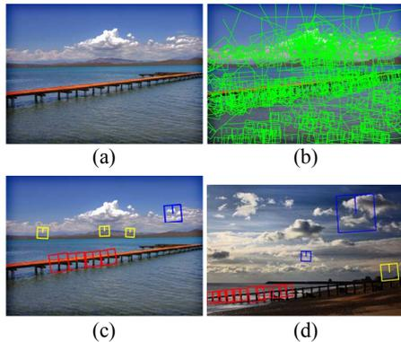
Figure 3: An illustration of the relationship between SIFT features and visual words. (a) A database image. (b) The extracted SIFT descriptors (highlighted with green boxes). (c)–(d) SIFT descriptors detected from two database images that are quantized into three visual words (highlighted in red, yellow and blue respectively).
