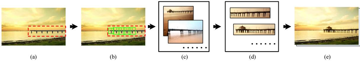
Figure 2: System overview. (a) A sketched target image. (b) The extracted SIFT descriptors from the sketched area (highlighted with green boxes). (c) Top ranked candidate images after the first-step ranking. (d) Top re-ranked candidate regions after the second-step re-ranking. (e) Compositing results.
