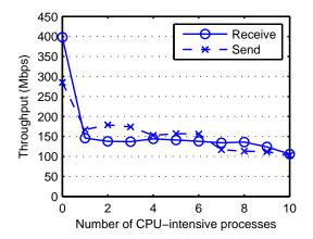
Figure 3: TCP throughput under high CPU load
