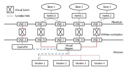
Figure 1: Network subsystem of a mobile PlanetLab node
