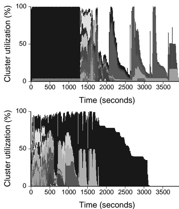
**Figure 7: Cluster utilization without and with preemption.** Shaded regions correspond to application instances, and their area indicates the number of running workers belonging to that instance. The top graph shows QF, with QFP below. The black region is PrimeLarge which occupies most of the cluster at the start and cannot be preempted by QF. QFP shares resources more fairly and completes sooner. Both stages of the final two iterations of PageRank are clearly visible in the lower plot.
