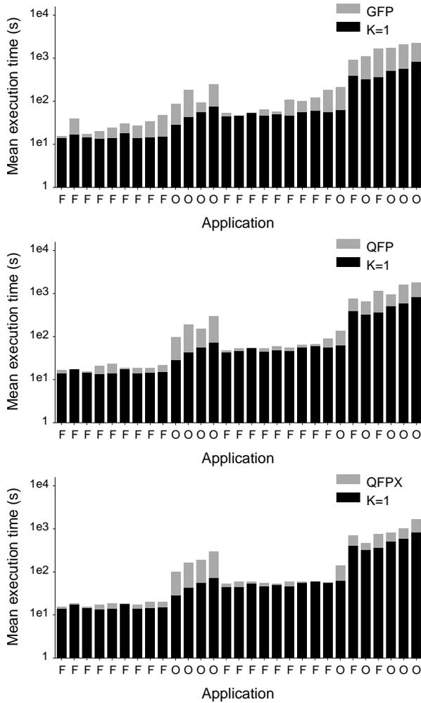
Figure 9: Average running time of each job for each policy using a constrained network with concurrency  $K = 10$ , compared to the ideal running time with  $K = 1$ . Labels on the horizontal axis are as in Figure 5.
