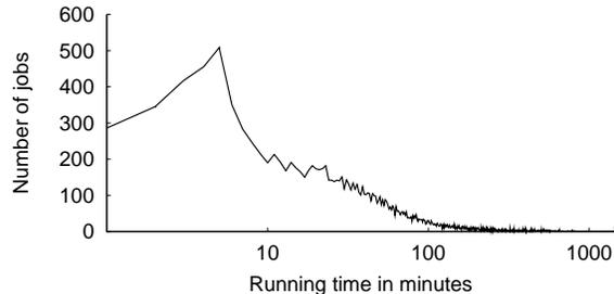
**Figure 1: Distribution of job running times from a production cluster used inside Microsoft's search division.** The horizontal axis shows the running time in minutes on a log scale, and the vertical axis shows the number of jobs with the corresponding running time.
