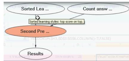
**Figure 3. Dependencies between to-do items (recall that their names are automatically generated and can be modified) are displayed in a directed graph: StratCel visualizes both within and between worksheet transitions.**
