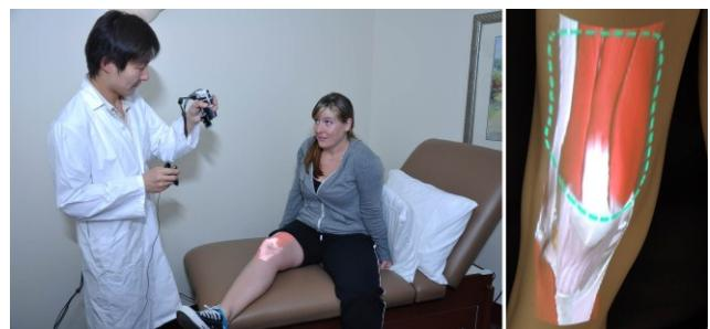
Figure 1: AnatOnMe in use in a simulated physical therapy consultation. The physical therapist explains a knee injury to his patient using on-body projection of medical imagery.
