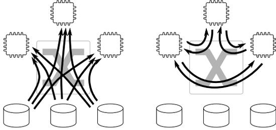
Figure 1: *Read phase*. In its reader role, each sort process (a) streams tracts, gathered by FDS from many tract-servers, from its part of the input file. It bins the records, and (b) transmits the bins to other sort processes acting the the bucket-receiver role.
