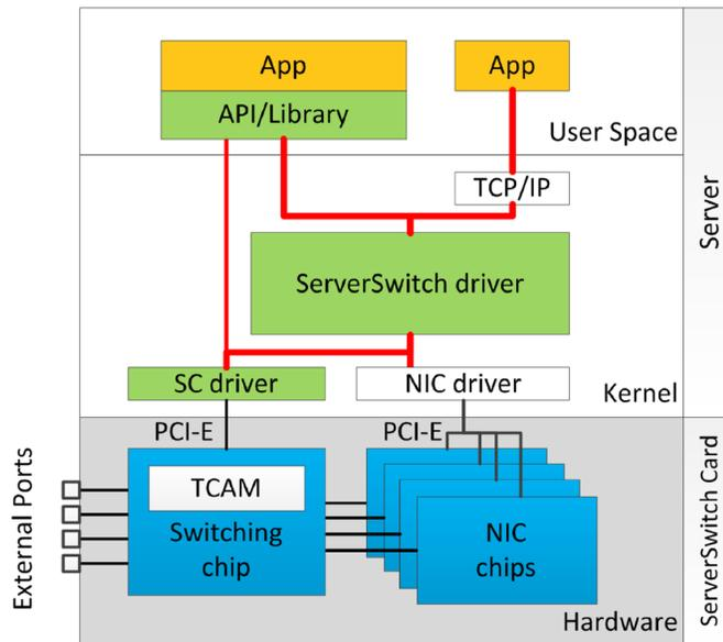
FIGURE 8: System architecture for ServerSwitch in [13].
