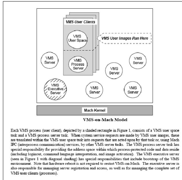
FIGURE 4: Digital Equipment's VMS on Mach Microkernel Prototype (Source: Wiecek et al [20])
