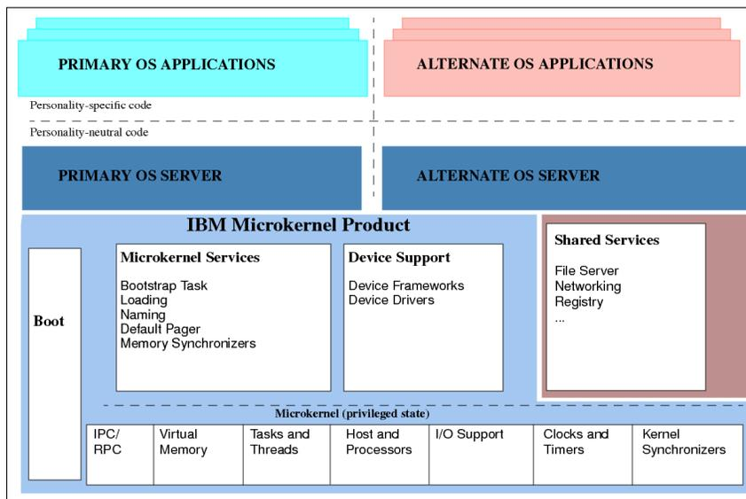
FIGURE 5: Structure of IBM's Workplace OS (Source: Rawson [18])
