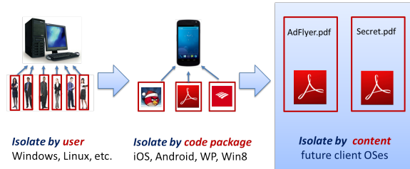
Figure 1: The evolution of isolation policies. Content-based isolation provides two benefits over other policies: (1) Any remote content’s impact is minimized (2) There is no need to ask users to determine whether to risk opening remote content.
