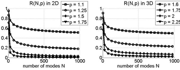
Fig. 3: Choosing  $N$ : The figures plot the residual ratio  $R(N, p)$  versus  $N$  for different  $p$  values in 2D (left) and in 3D (right). As expected the error upper bound drops with increasing  $N$ . The rate of decrease also becomes faster with increasing  $p$ . This inverse relation suggests the trade-off between  $N$  and the sensitivity of WESD to finer scale shape differences since WESD becomes less sensitive as  $p$  increases, see Section III-C.
