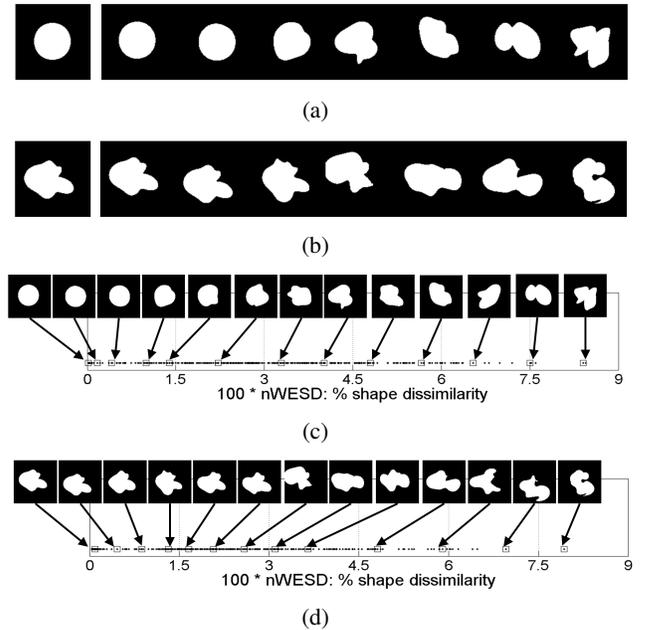
Fig. 4: Shape-based ordering of objects: We generate two artificial datasets each consisting of a reference object and its random deformations. Samples from the datasets are shown in (a) and (b). The binary images to the very left show the reference objects for each dataset. We then ordered all the deformed objects with respect to the nWESD scores between the object and the reference. The graphs in (c) and (d) plot these orderings. Based on visual inspection the ordering is quite reasonable.
