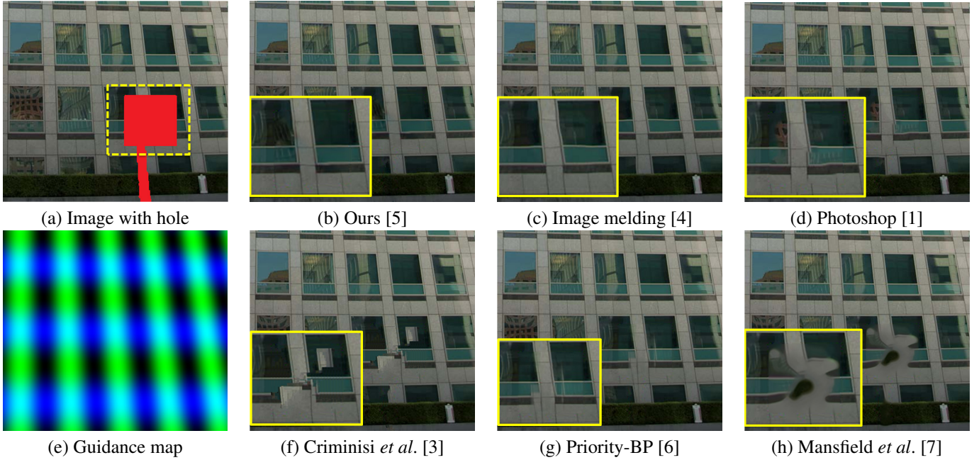
Figure 2. Image completion comparison (a) input image with a hole (marked as red), where visible parts contain rotational symmetry; (b) ours (with guidance map (e)) [5]; (c) Image Melding [4]; (d) Photoshop Content-Aware Fill [1]; (e) positional guidance map; (f) Criminisi et al. [3]; (g) Priority-BP [6]; (h) transforming image completion [7].
