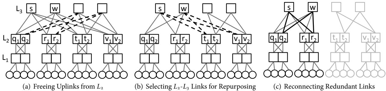
Figure 2: Modifying a 3-Level, 4-Port Fat Tree to Have 1-Fault Tolerance at  $L_3$
