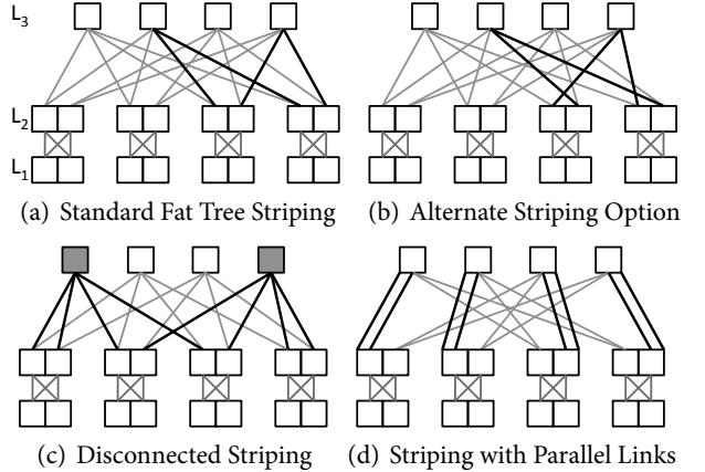
Figure 6: Striping Examples for a 3-Level, 4-Port Tree
