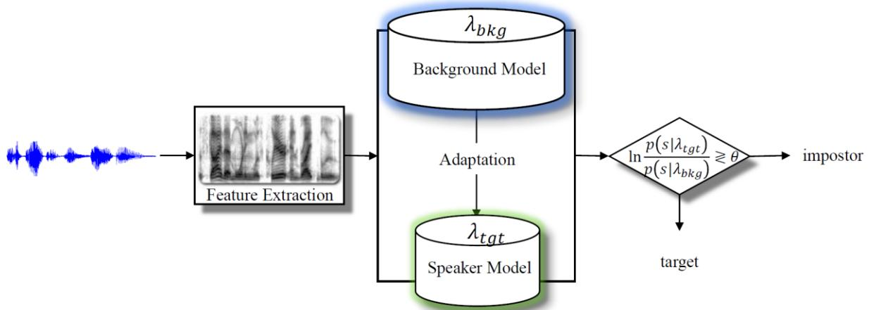
A speaker recognition system includes two primary components: a front-end and a back-end. The front-end transforms acoustic waveforms into more compact and less redundant representations called acoustic features. Cepstral features are most often used for speaker recognition. It is practical
