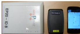
Figure 1. Hardware Prototypes anchor node “easyPoint”, tag “Rex” and mobile device with app
