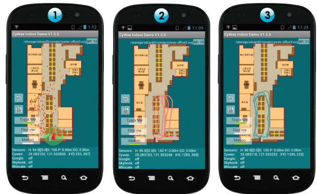
Figure 1: Indoor localization using solely WiFi (left), solely IMU (middle) and location fusion (right) while a user walks several times along a rectangular path in a typical office environment.
