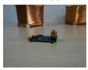
ter axes which are sequentially pulsed. 3 perpendicular coils on the receiver PCB measure the voltages induced by the oscillating magnetic fields. The voltage levels depend on the position of the receiver in the magnetic field and the orientation of the receiver. The transmitter and the receiver coil use oscillating circuits with a resonant frequency of 20kHz to maximize the field output and minimize electromagnetic distortions.
