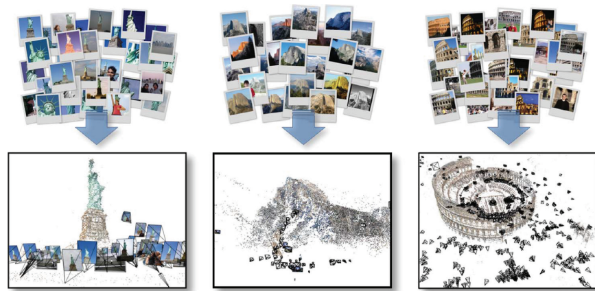
Fig. 1. The Photo Tourism system takes collections of Internet images (originally found using keyword search) and reconstructs a sparse 3D point model of the scene along with the camera locations associated with each photograph. This information can then be used to interactively browse the collection of photos.
