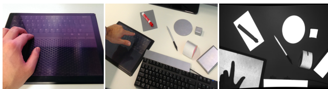
Figure 2: Left: passive retro-reflective keyboard, and series of other "physical widgets". Right: IR image of scene.
