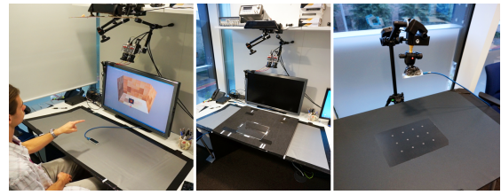
Figure 9: Study setup. Left: Kinect, Leap and RetroDepth setups for 3D acquisition task. Middle: Kinect touch evaluation. Right: Leap touch evaluation.
