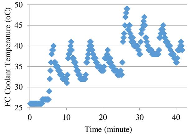
**Figure 7. The fuel cell coolant temperature profile during the series of step load changes.**
