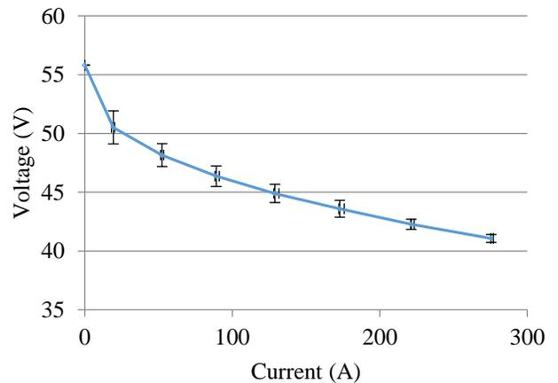
**Figure 2. Stack I-V polarization curve of the 12kW in-rack PEMFC system. Error bars in the data indicate ± one standard deviation from 5 different measurements.**
