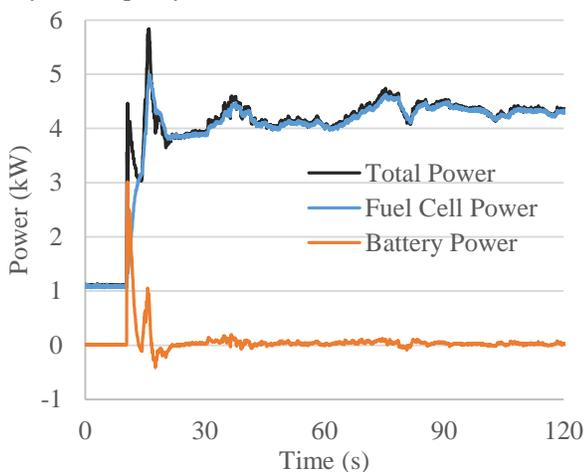
**Figure 10. The hybrid system transient responses to server dynamic operation, 9 servers were turned on at t=10.**
