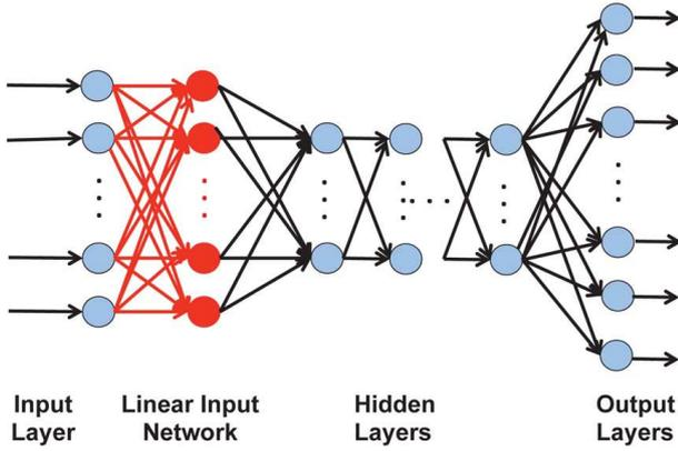
Figure 2: An architecture for adapting ANN-HMM models based on LIN. During adaptation, the parameters (weights) associated to the red links are estimated using the adaptation utterances while all other weights are kept fixed. The activation function for each LIN neuron (red node) is linear.
