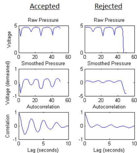
**Figure 3.** The accepted respiration signal(left) shows a much larger difference between the first valley and peak of the autocorrelation than the rejected signal (right).
