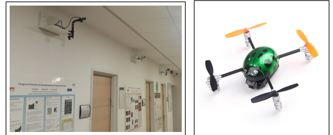
Figure 1: (left) 3 IoTracker clients installed near the ceiling of our CS department. (right) The RC lady-bird $30 quad-copter that we turned into IoTracker-based autonomous robot.
