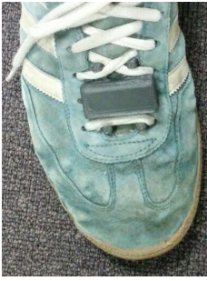
Figure 1: Top view of the foot sensor. Size is approximately 4x4x1cm
