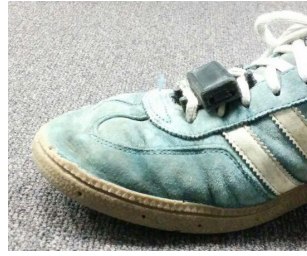
Figure 2: Side view of the foot sensor attached to the strings of a shoe.
