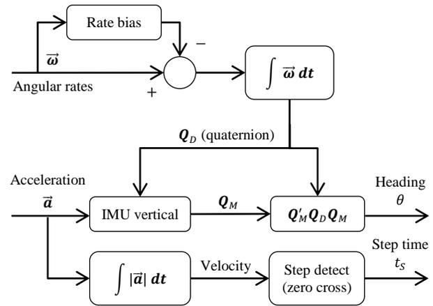
Figure 1. Inertial signal processing
