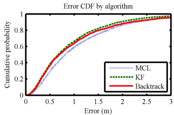
Figure 6. CDF of position error, by algorithm.
