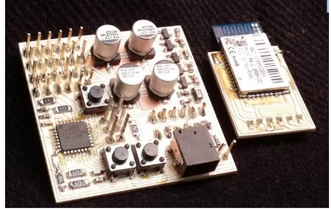
Figure 4: The above picture shows the Coordinator on the left and the Bluetooth module in the middle that attaches to the underside of the Coordinator.
