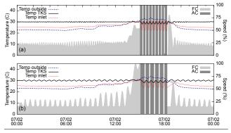
Figure 6. Real (a) and Real-Sim (b) baseline runs on 7/2/13.
