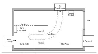
Figure 4. Internal layout of Parasol.
