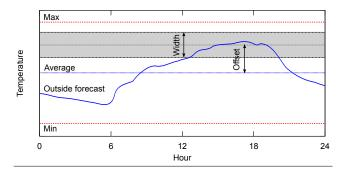
Figure 3. Temperature band selection in CoolAir.
