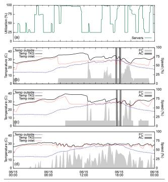
**Figure 7.** Workload (a), real (b), Real-Sim (c), and Smooth-Sim (d) CoolAir runs on 6/15/13.
