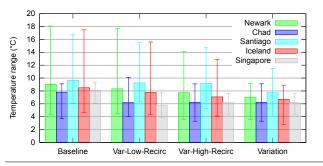
**Figure 11.** Temperature ranges, as a function of spatial placement and approach for limiting variation.
