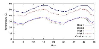
Figure 1. Disk, inlet, and outside temps under free cooling.
