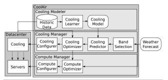
**Figure 2.** Architecture. Rectangles with square corners represent modules, whereas round corners represent derived or input data.
