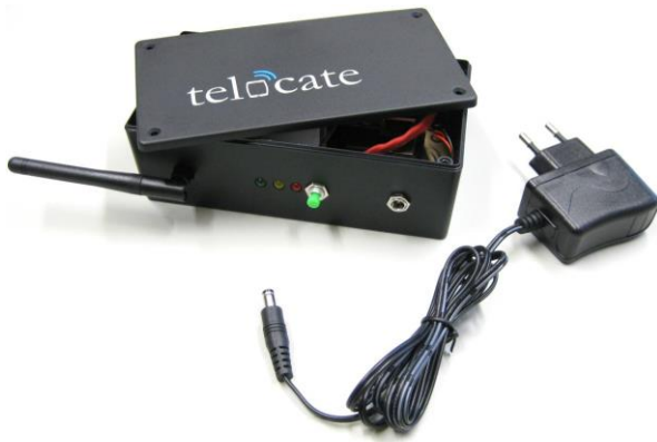
Fig. 2. Telocate custom made acoustic receiver
