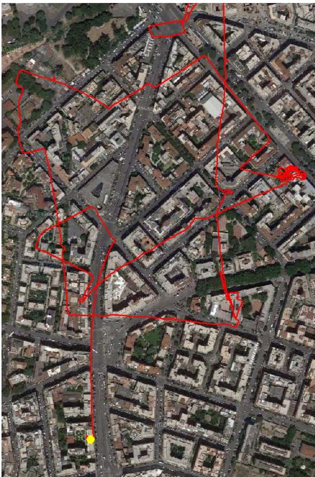
Fig. 1. Purely Inertial path estimated with a SoA PDR algorithm (5.300 m, 1h 49 m walk); no GPS or compass augmentation employed.
